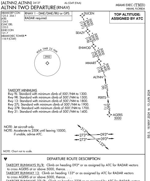
TAKEOFF RUNWAYS 27L/R: Climb on heading 273° or as assigned by ATC for RADAR vectors to cross AGERS at or above 5000, thence. . . .
