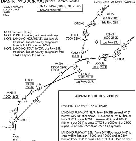
092° to cross JODUS at or above 7000 and at 220K, then on track 092° to CHIRM, then on track 054° to cross KENCH at 6000 and at 210K, then on track 054°. Expect RNAV (RNP) Z RWY 23L approach.
